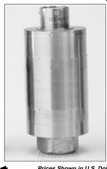
The OMEGADYNE™ PX32 Series is a rugged, high temperature transducer. Its hermetically sealed, all stainless steel construction and high temperature operating range make it ideal for measuring hydraulic pressure on industrial and off-road equipment or industrial applications where high temperatures are encountered. The PX32 is available in gage, absolute or sealed models. An environmentally sealed, twist loan connector is standard.
